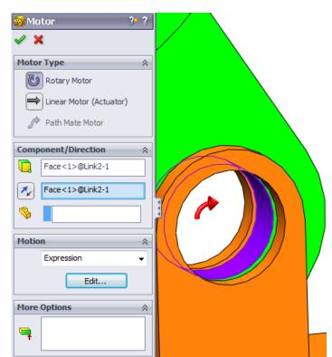
Note: The last field under Component/Direction property dialog, Component to more relative to, is used to specify reference component for the relative motion input. Since we wish to move Link2 with respect to the fixed Base, this field will be left blank.
