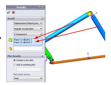
The plot shows the acceleration magnitude of Link1 (its center of mass) with respect to Link3 (part's coordinate system). The maximum relative acceleration is 139 deg/sec^2 in the negative rotational Z direction.
