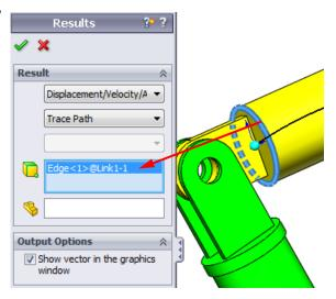
**Note:** The resulting trace path is by default shown with respect to the fixed ground. To show the trace path with respect to another moving component, one would have to select this reference component as a second item in the same selection field.
