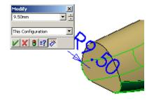
By increasing the radius value the curves of the body will be smoother both at the front and along the length of the body.
