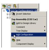
However, the new configuration is identical to the Default configuration. We need to change it so that this configuration shows the modified car body.
