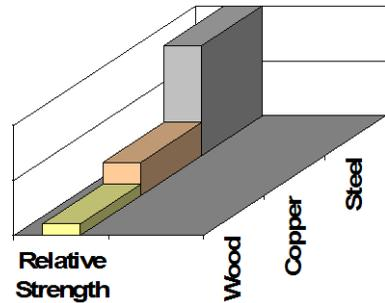
**Note:** Metals are manufactured products and due to the way they are created, they have equal strength in each direction. Materials like this are called *isotropic* materials.
