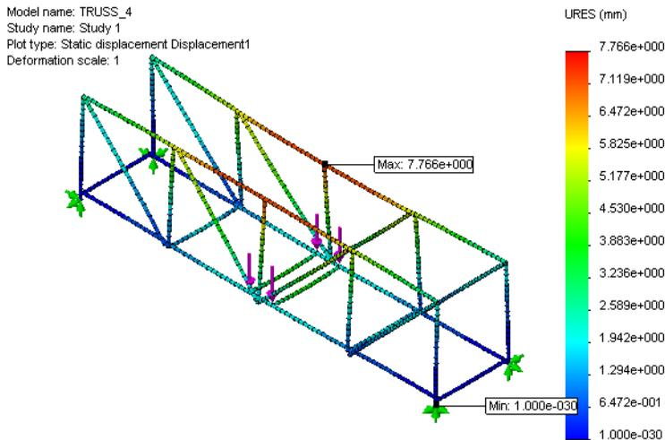
The displacements are small but you may notice that the model seems oddly shaped. The upper portions of the walls are bending inward. Some additional bracing is required.
