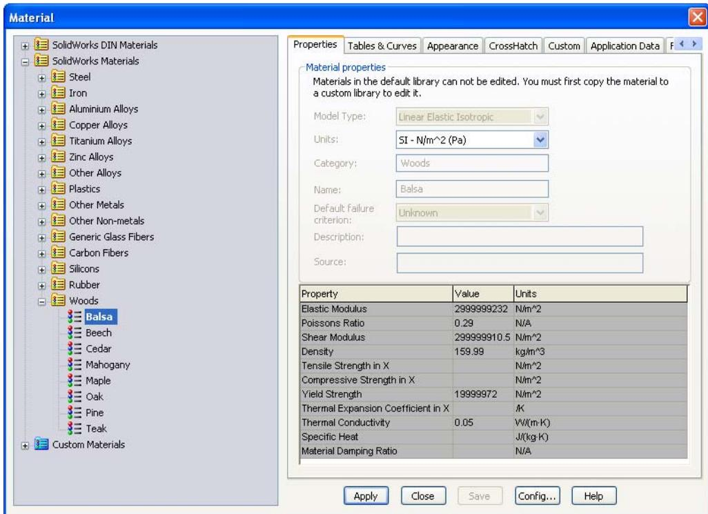
**Note:** The material used, **Balsa**, is chosen to make the analysis useful to those who will actually design, construct and test the structure. Balsa wood is a common material for student building projects.
