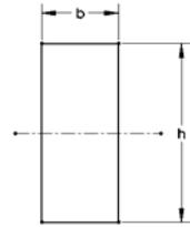
The Area Moment of Inertia is used in calculations as resistance of a beam to bending. The higher the value, the more resistance against bending.
