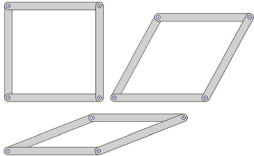
Adding a 5th member diagonally makes a big difference. The shape is now locked in that position. The addition has broken the parallelogram into two triangles.
