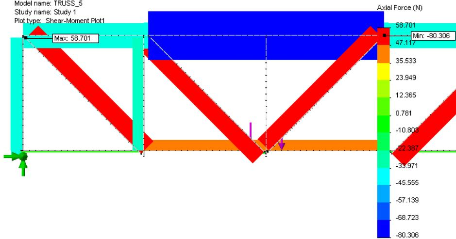
**Note:** The axial forces in the vertical member nearest the external loads are very small because the braces absorb most of the load.
