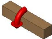
A 3D perspective view of a brown rectangular beam. A red curved arrow is shown around the beam, indicating torque.                                 |
