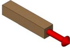
A 3D perspective view of a brown rectangular beam. A red arrow points along the length of the beam, indicating axial force.                          |
