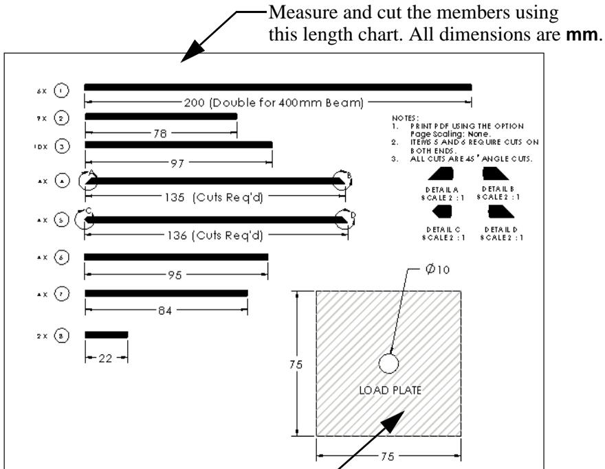
Cut out this Load Plate shape to test the inside width of your structure.
