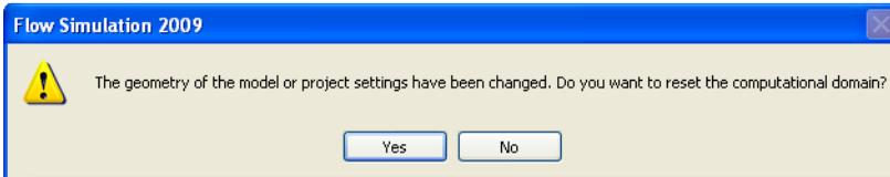
The system will ask you if you want to reset the computational domain. Click **No**. To make it easier to do meaningful comparisons between the two sets of results, we want to use the same size computational domain. Also, resetting the domain would require us to redefine the symmetry conditions. That would be extra work.
