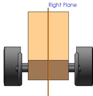
2. In this model we use half symmetry, therefore any forces you calculate will have to be doubled. For example, the magnitude of the force that represents drag on the car is actually only half the total force because only half of the car is analyzed.
