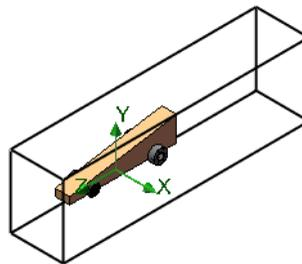
**Note:** Reducing the size of our computational domain and utilizing a symmetry boundary condition will allow for more efficient calculations. We must always be sure, however, that our computational domain is large enough to allow our flow field to fully develop.
