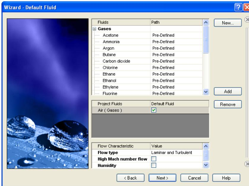
**Note:** Flow Simulation has a database library of several liquids and gases which is called the Engineering Database. With this database you can create your own materials.
