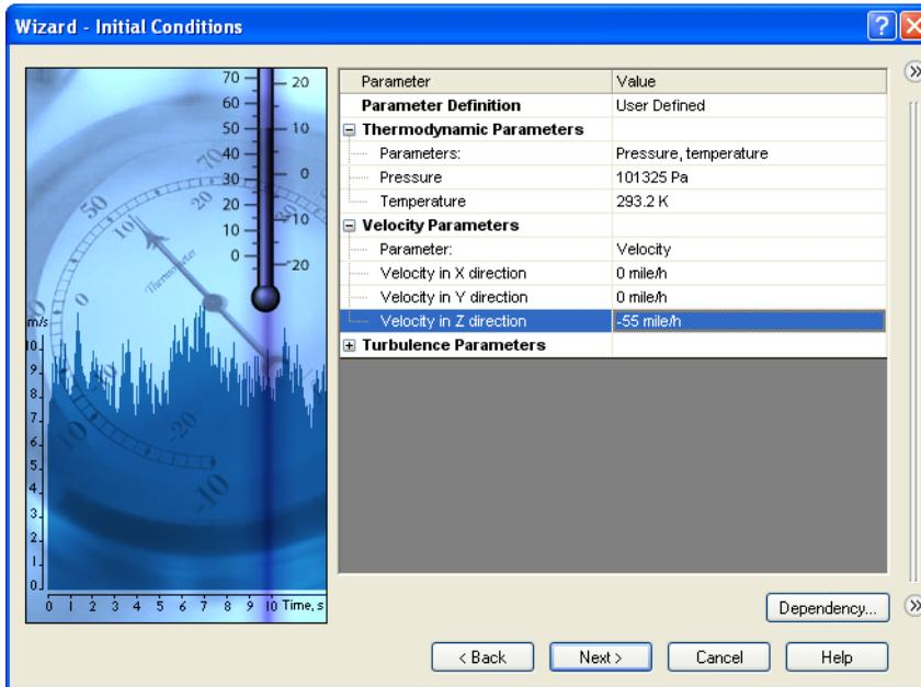
In the real world, the car would be moving through stationary air. In a wind tunnel, the car is stationary and the air is moving. You can think of this Flow Simulation example as a virtual wind tunnel – the car is stationary and the air is moving.
