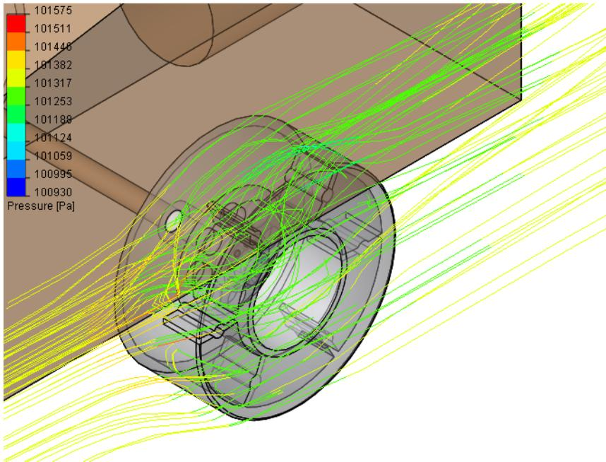
It is now easier to see the turbulence in the airflow between the wheel and car body.
