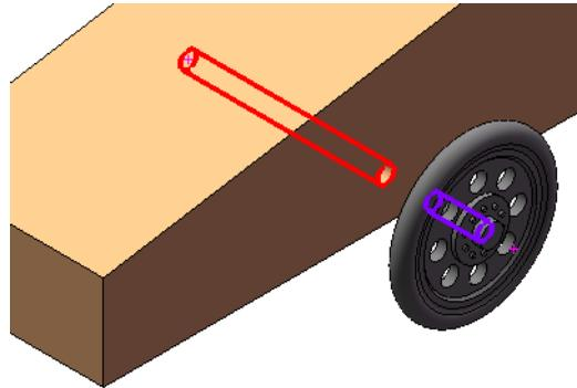
However, this is not the best strategy. A **Coincident** mate requires two planes, either faces or reference planes. If we modify the shape of the car body so that the side is no longer planar, then the **Coincident** mate will fail.
