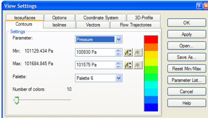
**Note:** The reason we do not use the default values is because if we make a design change to the car and rerun the analysis, the minimum and maximum pressure values will be different. That means red would represent one pressure on one plot and a different pressure on a different plot. Using the same minimum and maximum settings for each analysis allows for meaningful comparisons between different iterations of the design.
