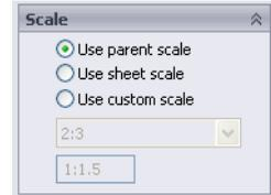
The views that were projected off of the first view are linked to the scale of the source or parent view.
