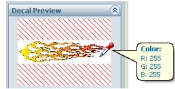
That means, any pixels in the decal which have the selected color will be treated as transparent.
