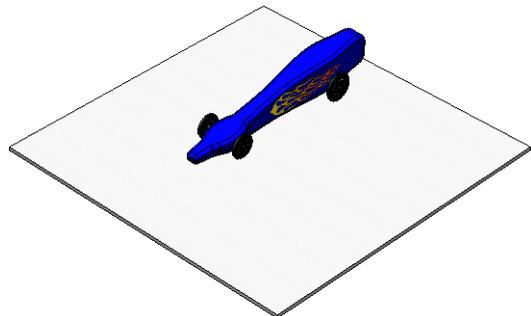
Add a **Parallel** mate between the **Top** reference plane of the **Floor** and the **Top** reference plane of the assembly. This will keep the **Floor** from tilting.
