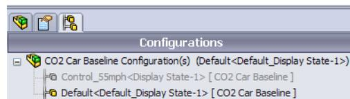
The Flow Simulation analysis tree tab
