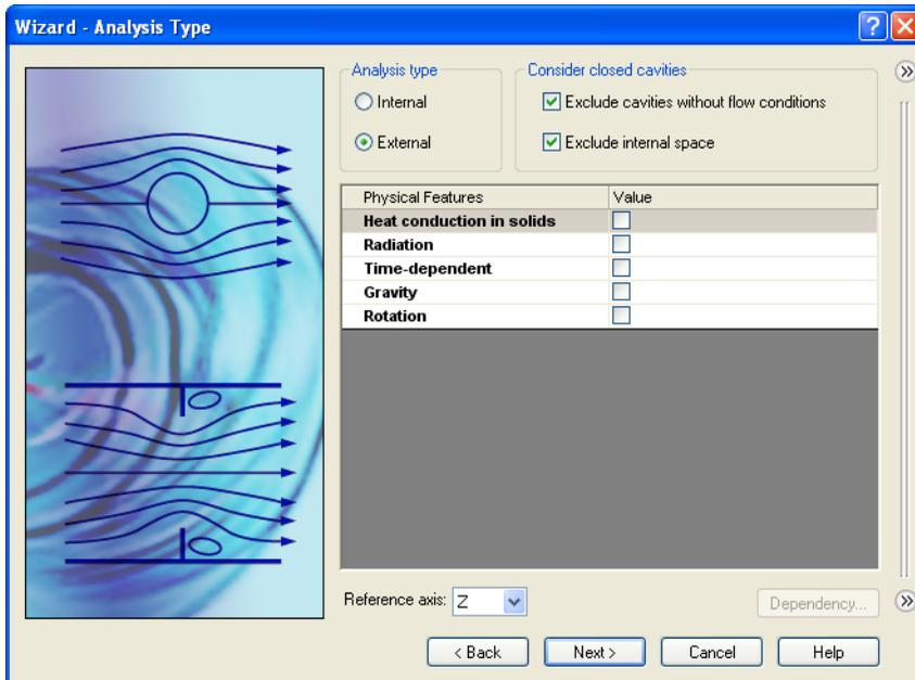
**Note:** An internal analysis examines enclosed flow pathways while an external analysis examines open flow paths. You would use an internal analysis for something like an exhaust manifold for an automobile engine.
