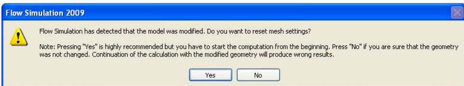
The geometry of the car body has changed. We've rounded the nose and made other changes. The mesh should be reset.
