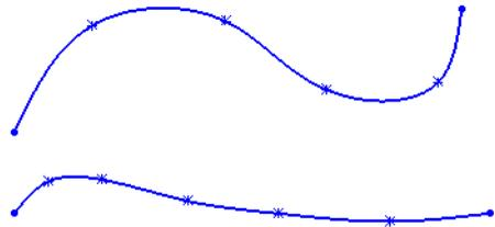
You can modify a spline by adding or deleting points, moving the points, dimensioning the points, changing tangency at the points, or adding geometric relations.
