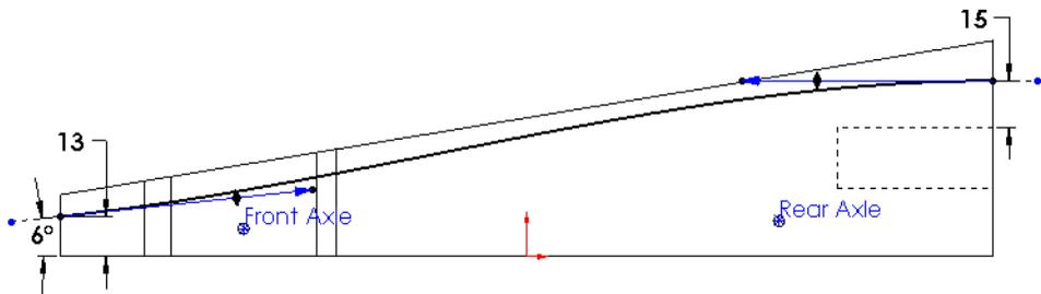
**40 Adjust the length of the spline handles.**
