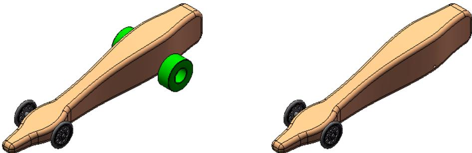
The wheels along with their mates are suppressed. They aren't deleted from the assembly, they are just "turned off". They will not be included in any system calculations.
