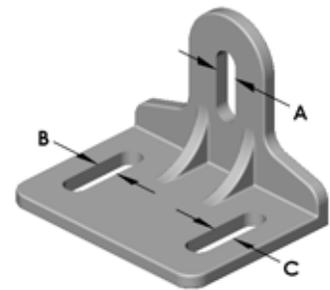
**Answer:** You should use **Link Values**. An **Equal** geometric relation will not work because **Equal** only works inside a sketch. Features A, B, and C cannot be in the same sketch.
