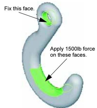
Follow the instructions in *Design Analysis: SolidWorks SimulationXpress: Using Analysis to Save Material* in the SolidWorks Tutorials. In this lesson, you use the results from SolidWorks SimulationXpress to reduce the volume of a part.
