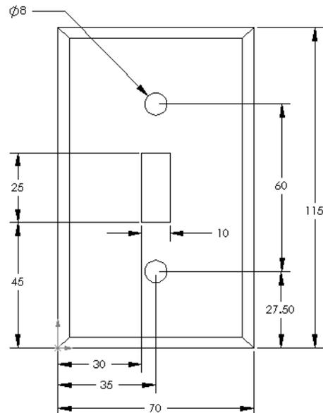
5 Create a simple single light switch cover using SolidWorks. The filename for the part is switchplate.
