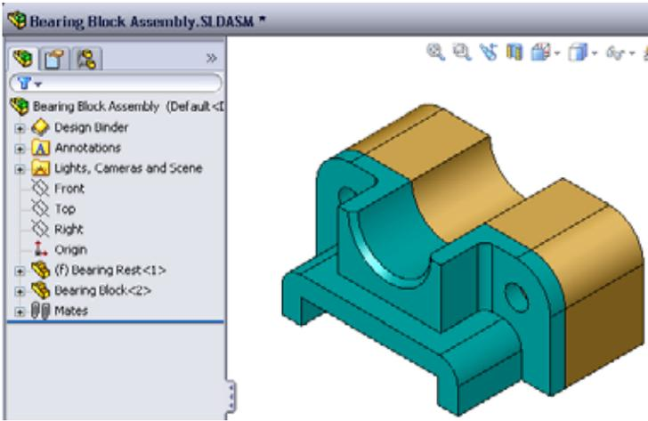
the bearing block are tapped holes. Tapped holes are threaded and specifically designed to act like nuts do. In other words, the bolt screws directly into the bearing block.
