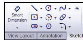
**2 Insert two Dimensions into the Front view.**
