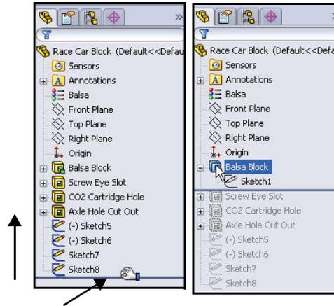
**Note:** The Balsa Block is 223mm x 50mm x 65mm. If you plan to use a fixture to machine your car, you must make sure that your design is no longer than 210mm. Most fixtures have a nose plate that holds the front of the balsa block and if your design is too long, it can/will end up breaking the endmill or possibly damaging the fixture.
