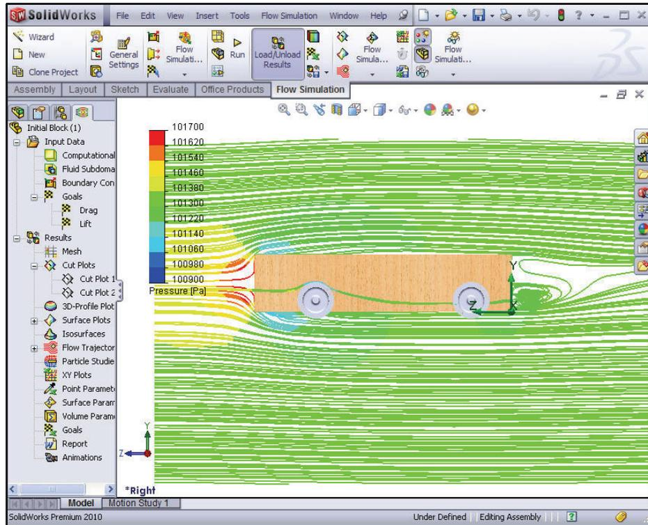
**Note:** Notice the turbulence in front and behind the body of the block.
