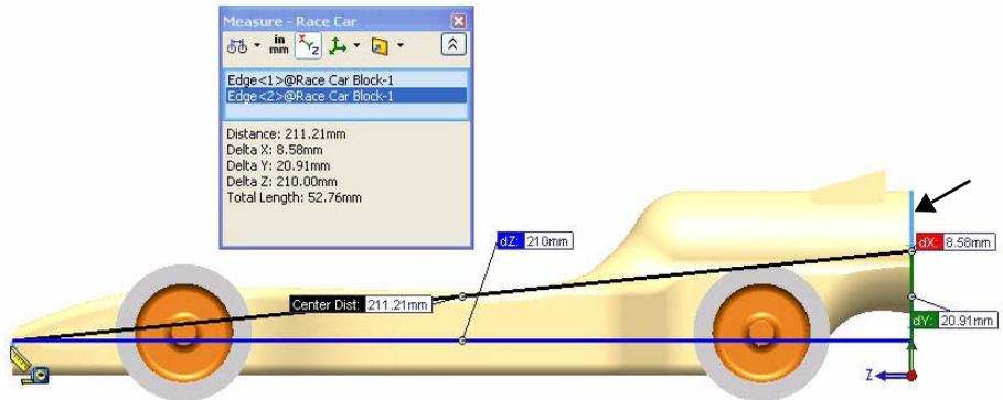
**Note:** The Balsa Block is 223mm x 50mm x 65mm. If you plan to use a fixture to machine your car, you must make sure that your design is no longer than 210mm. Most fixtures have a nose plate that holds the front of the Balsa Block and if your design is too long, it can/will end up breaking the endmill or possibly damaging the fixture.
