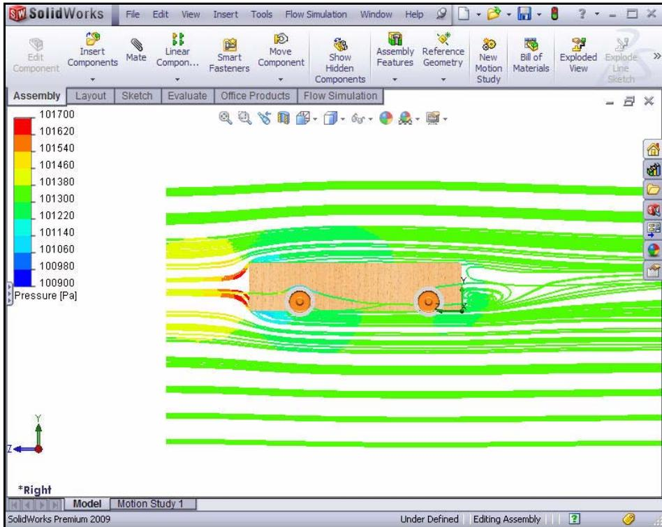
**Note:** Notice the turbulence in front and behind the body of the block.
