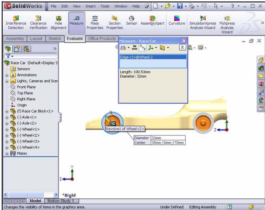
**3 Measure the center distance between the two Wheel hubs.**
