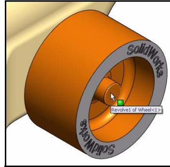
**3 Mate the three remaining Wheels to the Front and Rear Axles.**
