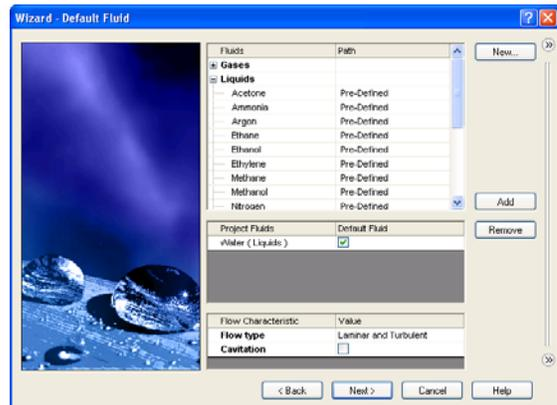
**Note:** The SolidWorks Flow Simulation **Engineering Database** contains physical properties of predefined and user-defined gases, real gases, incompressible liquids, non-Newtonian liquids, compressible liquids, solid substances and porous materials. It includes both constant values and tabular dependencies of various physical parameters on temperature and pressure.
