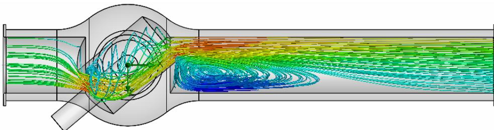
Some may prefer to display the flow trajectories with the help of a section plot. Use **Plane2** to define a section plot to show the flow trajectories.
