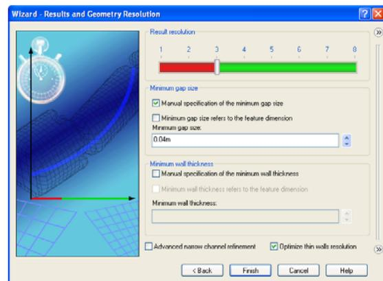
Select the **Manual specification of the minimum gap size** check box and enter **0.04 m** for the minimum flow passage.
