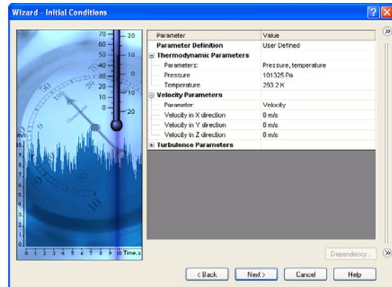
**Note:** For steady flow problems SolidWorks Flow Simulation iterates until the solution converges. For unsteady (transient, or time-dependent) problems SolidWorks Flow Simulation marches in time for a period you specify.
