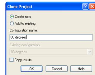
Now the new SolidWorks Flow Simulation project is attached to the new 00 degrees configuration and has inherited all the settings from the 40 degrees project. All our input data are copied, so we do not need to redefine them. All changes will only be applied to this new configuration, not affecting the old project and its results.
