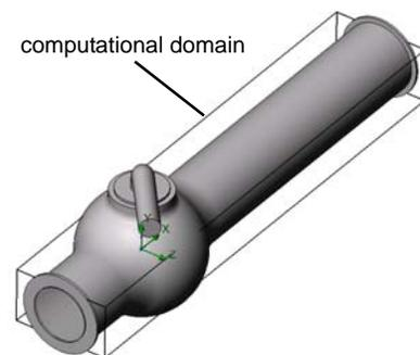
The next step is the specification of the boundary conditions. Boundary conditions are used to specify the fluid characteristics at the model inlets and outlets in an internal flow analysis or on model surfaces in an external flow analysis.
