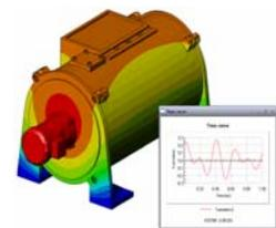
Motion Simulation enables user to analyze the kinematic and dynamic behavior of the mechanisms. Joint and inertial forces can subsequently be transferred into SolidWorks Simulation studies to continue with the stress analysis. Typical questions that will be answered using this modulus are:
