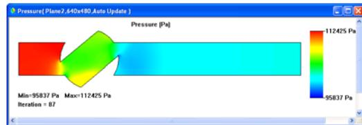
At the start of the run the results might look odd or change abruptly. However, as the run progresses these changes will lessen and the results will settle in on a converged solution. The result can be displayed either in contours, isolines or vector representation.
