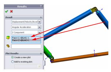
The plot shows the acceleration magnitude of Link1 (its center of mass) with respect to Link3 (again, its center of mass). The maximum relative acceleration is 139 deg/sec^2 in the negative Z rotational direction.
