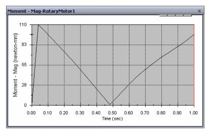
The required torque is about 110 N-mm
