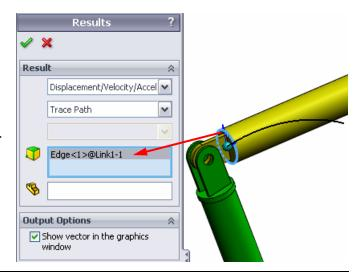
**Note:** The resulting trace path is by default shown with respect to the fixed ground. To show the trace path with respect to another moving component, one would have to select this reference component as a second item in the same selection field.
