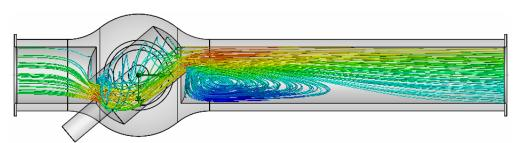
Some may prefer to display the flow trajectories with the help of a section plot. Use Plane2 to define a section plot to show the flow trajectories.
