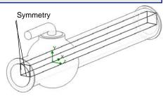
**Note:** The symmetric conditions can be applied only if you are sure that the flow is symmetric. Note that sometimes symmetry of both the model and the incoming flow does not guarantee symmetry in other flow regions, e.g. a von Karman vortex street behind a cylinder. In our case, the flow in the straight pipe is symmetric so we can reduce the computational domain.
