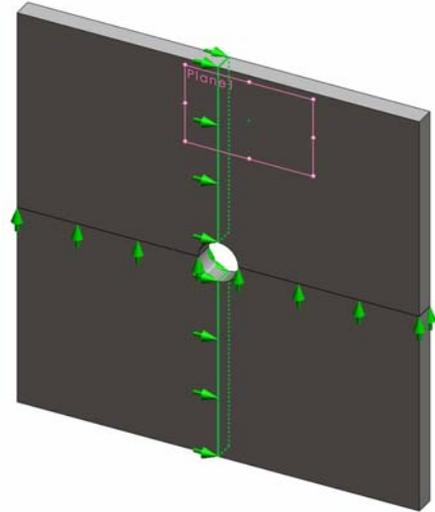
To prevent displacement of the model in the global Z-direction, a fixture on the vertex shown in the figure below must be defined.
