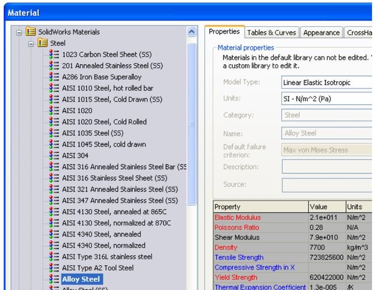
**Note:** The mechanical and physical properties of Alloy Steel appear in the table to the right.
