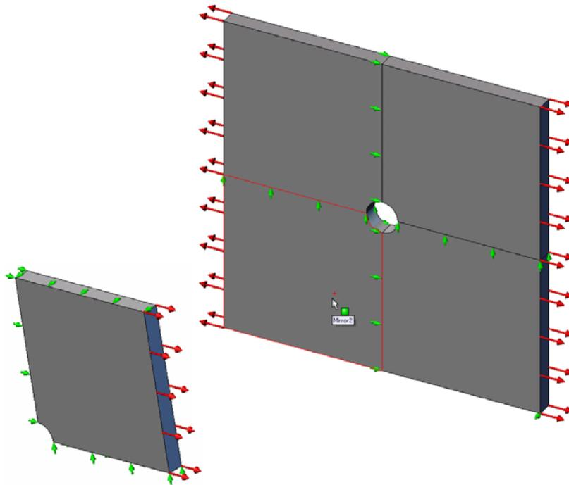
You will calculate the stresses of a 20 in x 20 in x 1 in square plate with a 1 inch radius hole at its center. The plate is subjected to a 100 psi tensile pressure.
