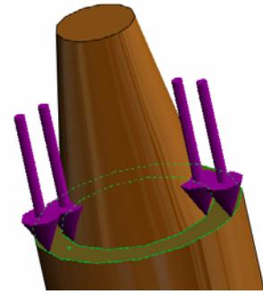
SolidWorks Simulation applies the force to the selected face and Force-1 item appears in the `External Loads` folder.
